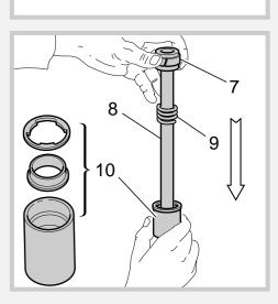
Reassemble the foot buffer (12) onto the end part of pumping rod (8).
